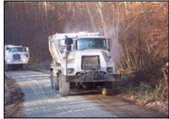
Mt. Carmel's custom built spreader trucks apply the cement on the subgrade at the prescribed application rate. These trucks are designed and built by Mt. Carmel personnel to meet precise standards for spreading accuracy, durability and dust control.
