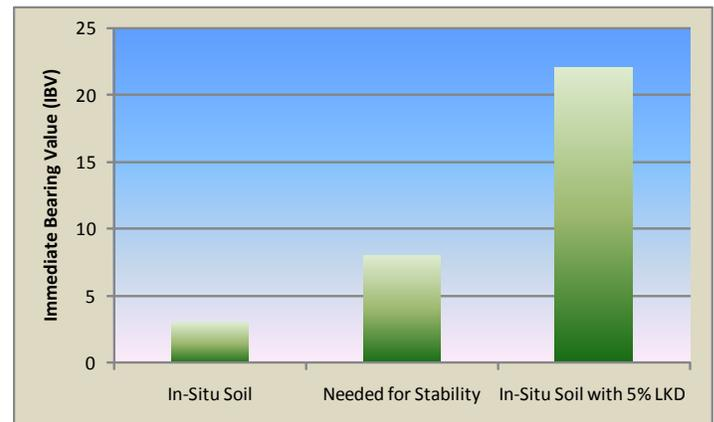
Chart 1 - Immediate Bearing Value (IBV) of soil before and after adding lime kiln dust.
