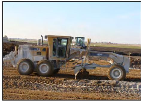
The motor grader shapes the area to rough grade.
